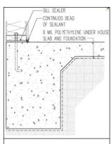
MONOLITHIC SLAB DETAIL
